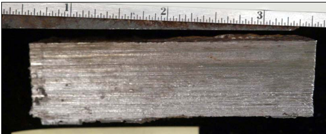
Figure 5.67. Cross section photograph of steel hull sample #USAR-02-006.
