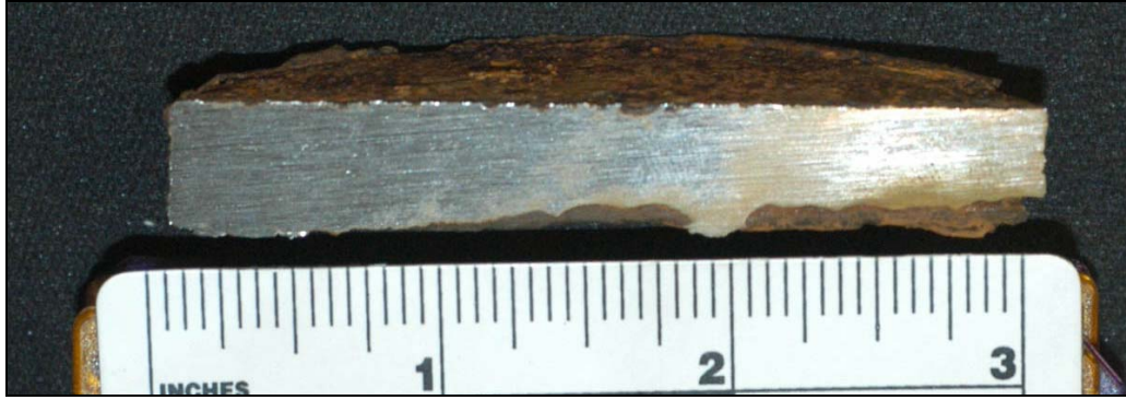
Figure 5.68. Cross section photograph of steel hull sample #USAR-02-007.
