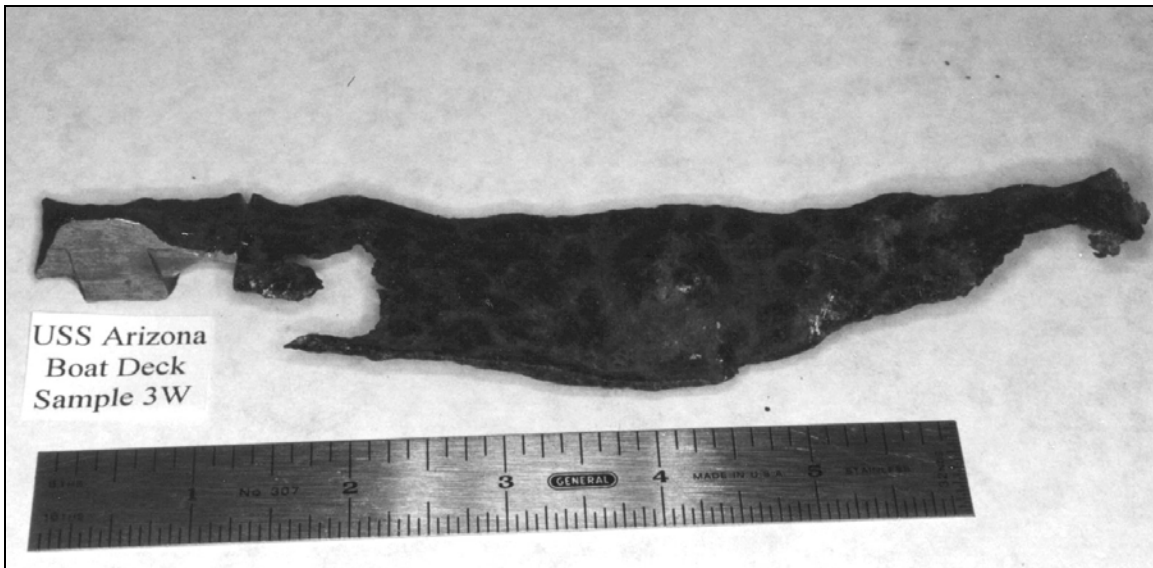
Figure 5.6. Sample W3, section with rivet in place from boat deck.
