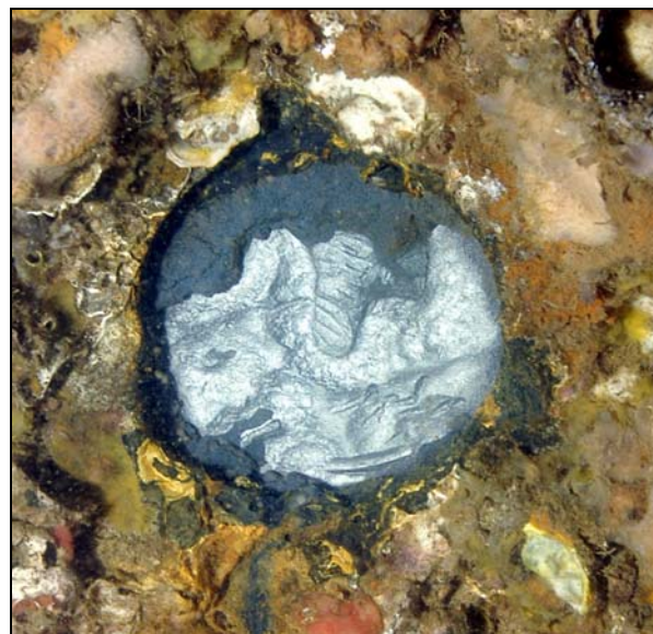
Figure 5.74. Steel surface of Arizona’s hull after extensive preparation. Part of the strongly adhering layer below the concretion remains at top. Uneven steel surface is due to corrosion (NPS Photo by Brett Seymour).
