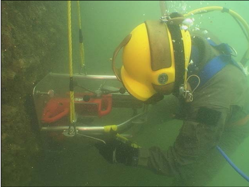
Figure 5.59. U.S. Navy diver using Titan’s hydraulic hole-saw to remove samples from Arizona’s hull (NPS Photo by Brett Seymour).
