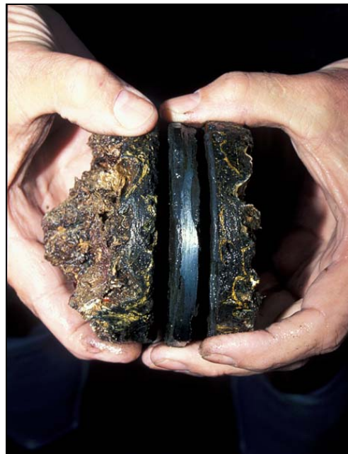
Figure 5.60. Steel hull sample with intact interior and exterior concretion (NPS Photo by Brett Seymour).
