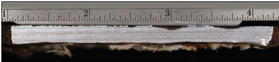
Figure 5.66. Cross section photograph of steel hull sample #USAR-02-005.
