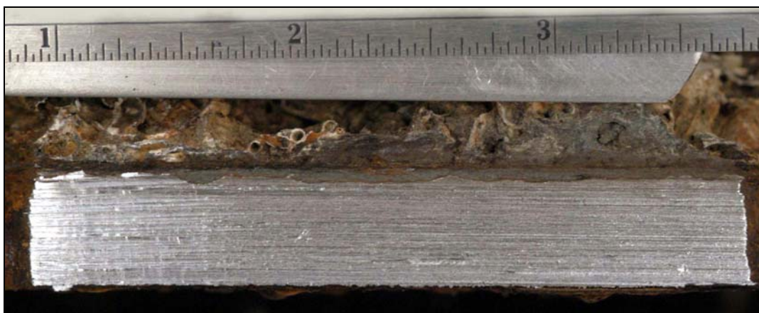
Figure 5.64. Cross section photograph of steel hull sample #USAR-02-003.
